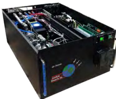
Figure 3. Picture (left, instrument top off) of the Aerodyne mini-TILDAS HCN monitor.
