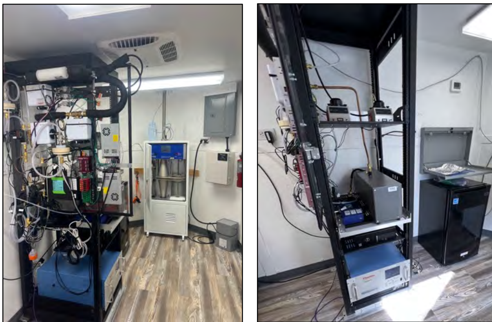
Figure 7. Left: Side view of the instrumentation and high-volume aerosol sampler. Right: Two tricolor absorption photometers (TAPs) and a nephelometer
